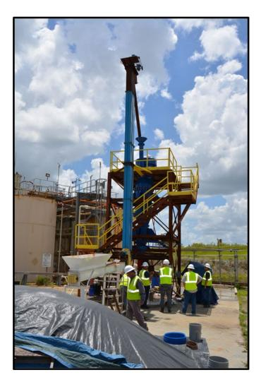
The Packed Column Jig pilot plant structure installed and functioning.
