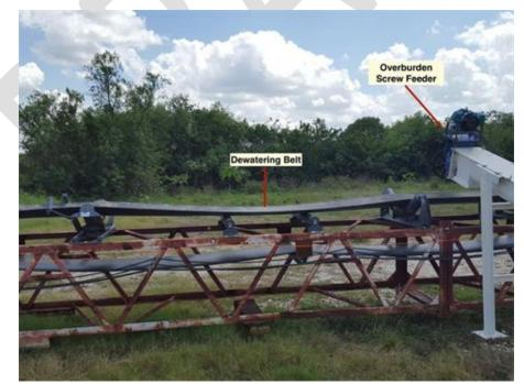
Overburden Screw Feeder and Dewatering Belt.
