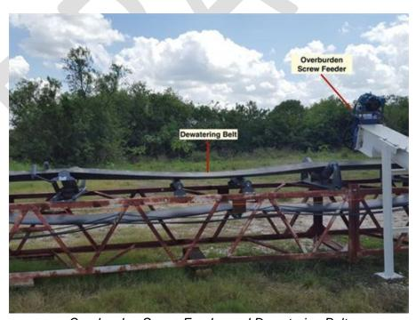
Overburden Screw Feeder and Dewatering Belt.
