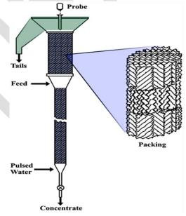
Components of the Packed Column Jig.
