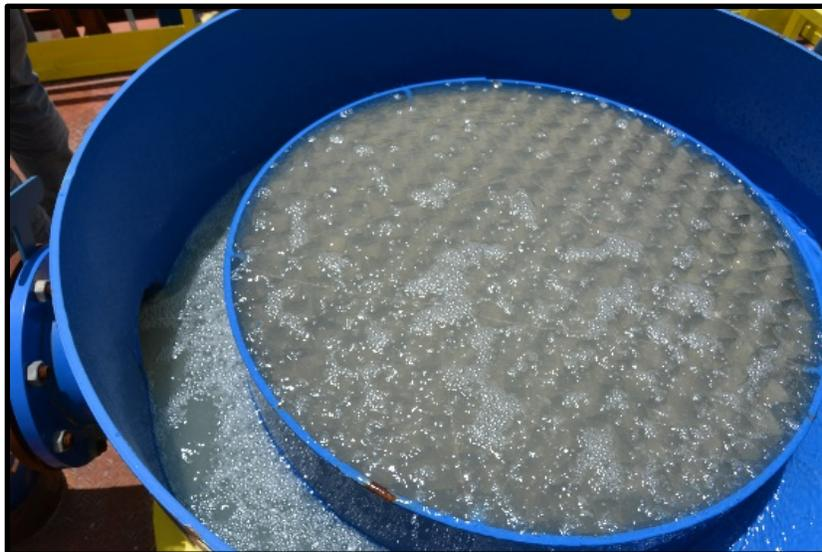
*View from the top of the jig column; water pushes up and fine particles move out with the wash-over.*
