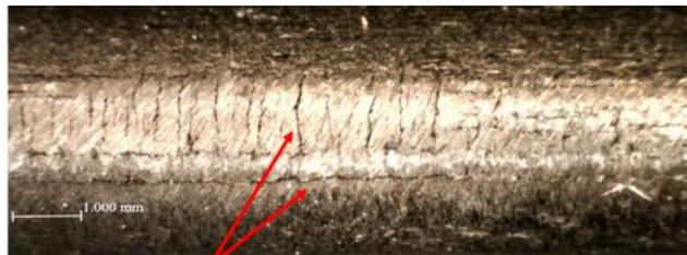
Fatigue cracks through and across build layers (X, Y and XY45)
