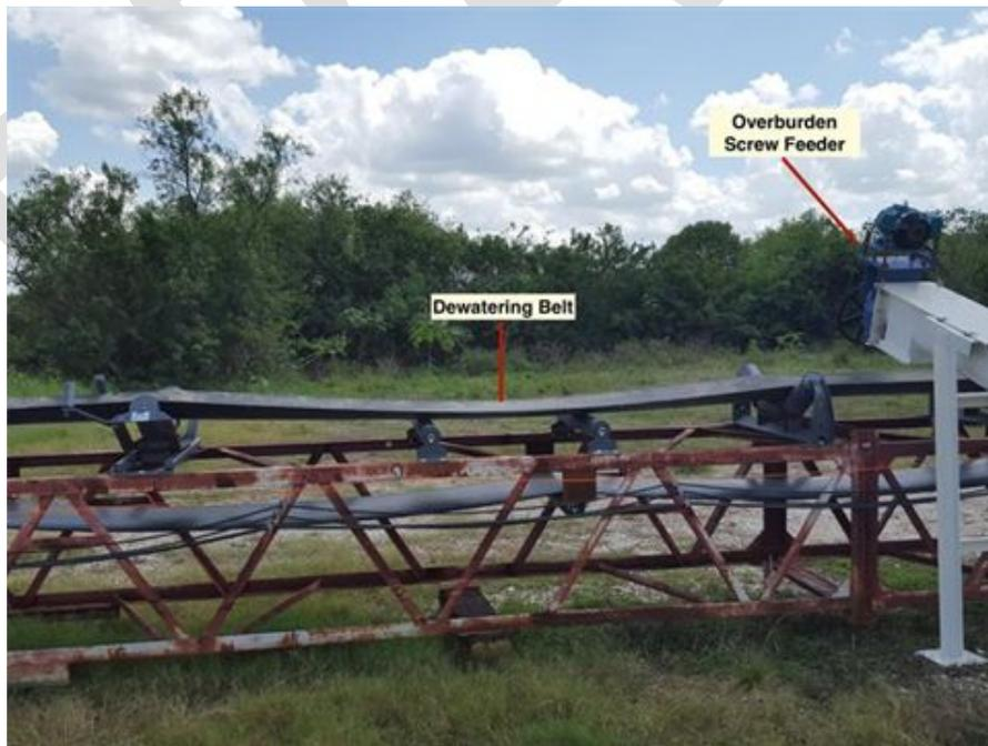
*Overburden Screw Feeder and Dewatering Belt.*
