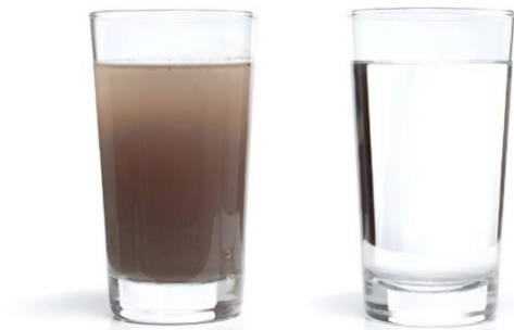
Figure 2: Example- A sample of the polluted water (left) can be compared to the filtered water sample (right) to determine with the naked eye if the turbidity of the sample has been reduced.
